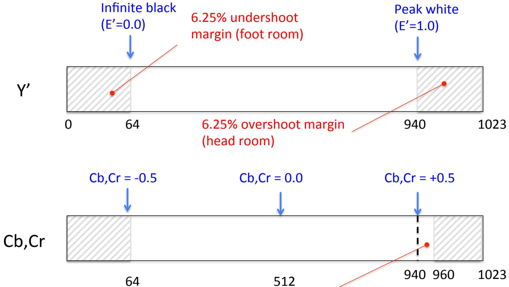
*A little extra legal range for Cb,Cr positive signals designed by original 1980's ITU-R (CCIR Rec.) BT.601 team to accommodate for saturated colors*
