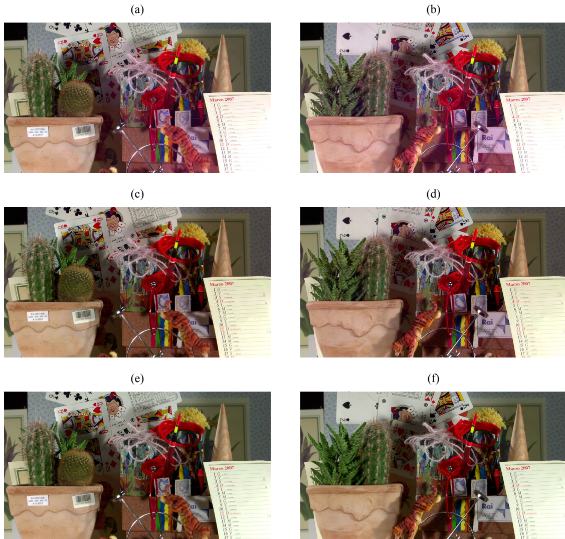
Figure 3 – Typical distortion introduced by 8-bit decoding of 10-bit sequences. Sequence cactus QP=27, first frame (left), last frame (right). (a,b) Method-1, (c,d) Method-2, (e,f) HM-10.
