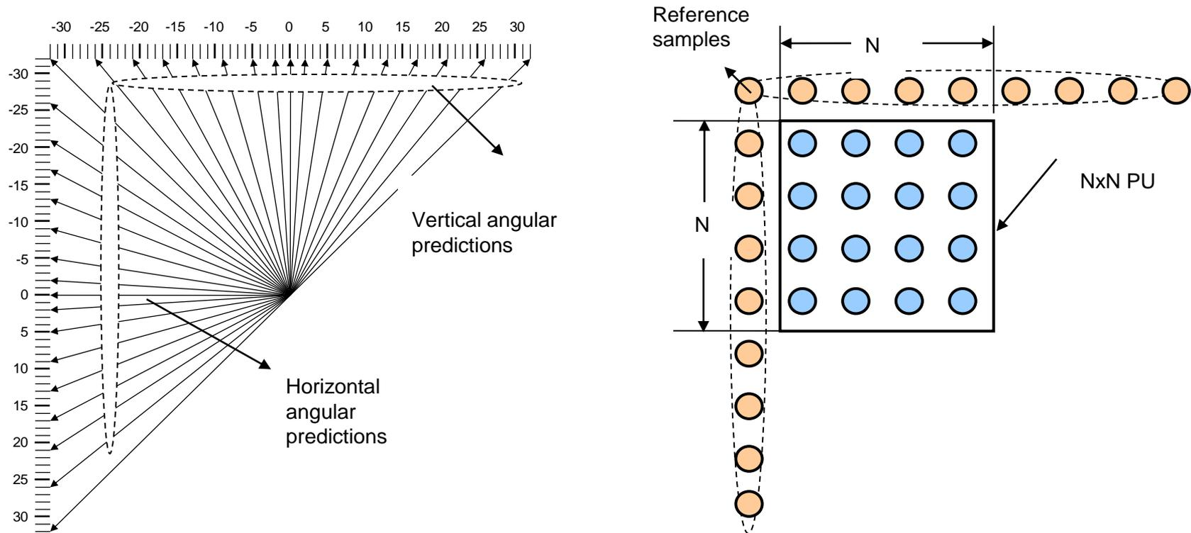
In lossless mode, not only the reference samples from neighboring PUs, but also the neighboring samples inside the current PU are available for prediction
