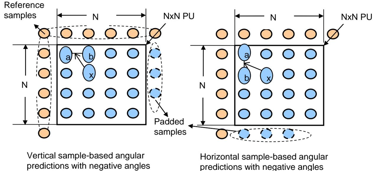
2. After the reference samples are determined, the same bilinear interpolation is used for generating prediction sample
