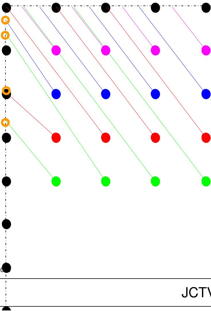
When side reference is used, pixels along a row (e.g. green pixels) use same deltaFract leading to warping in prediction signal when prediction is from side reference samples (in main reference array)
