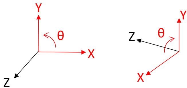
$$R_Z(pitch) = \begin{bmatrix} x \\ y \\ z \end{bmatrix} = \begin{bmatrix} \cos(pitch) & -\sin(pitch) & 0 \\ \sin(pitch) & \cos(pitch) & 0 \\ 0 & 0 & 1 \end{bmatrix} \begin{bmatrix} x \\ y \\ z \end{bmatrix}$$
