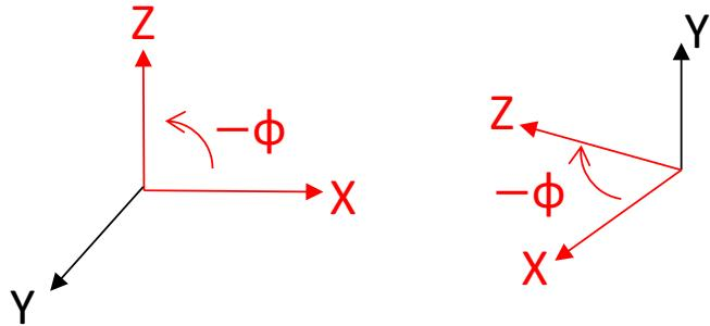
$$R_Y(yaw) = \begin{bmatrix} x \\ y \\ z \end{bmatrix} = \begin{bmatrix} \cos(yaw) & 0 & \sin(yaw) \\ 0 & 1 & 0 \\ -\sin(yaw) & 0 & \cos(yaw) \end{bmatrix} \begin{bmatrix} x \\ y \\ z \end{bmatrix}$$
